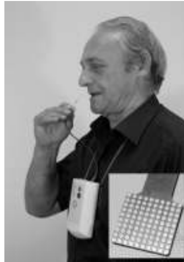
Fig. 1. The BrainPort Balance Device. Electrode Array.
